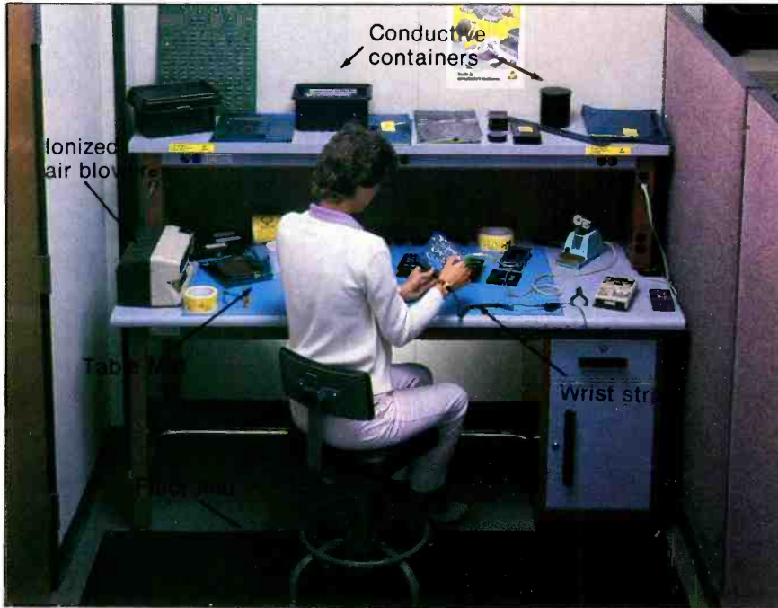
A typical static-protected work station includes mats, wrist straps and an ionized air blower.
