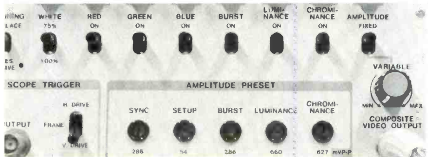
Figure 7. This generator permits front-panel adjustment of sync, setup, burst, luminance and chrominance amplitudes. Setup can be reduced to zero.
